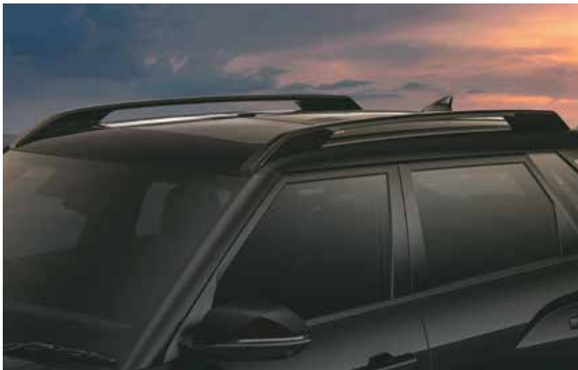
Black painted bridge type roof rails
